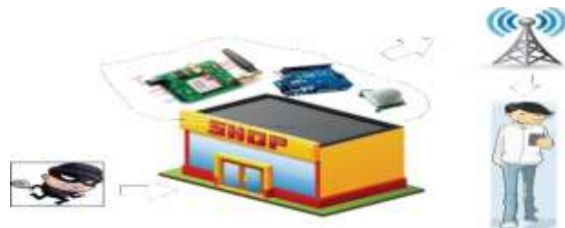
Figure 1. Space Security System uses a motion sensor with Arduino based SMS notification
