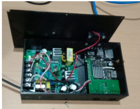
Fig. 6. Kiln Machine OCR Prototype
